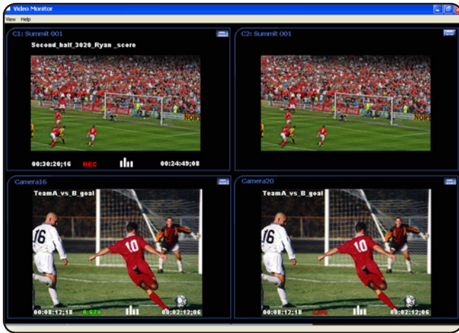
Internal multiviewer output on VGA provides a display of up to eight channels in real time when used with ChannelFlex.
