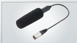
AG-MC200G XLR Microphone • Sensitivity: -40 dB ±3.5 dB (0dB=1V/Pa, at 1kHz) • Maximum Input level: 127 dB (1000Hz, Distortion within 1%) • S/N: More than 69 dB
