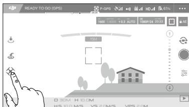
3. Tap once on the target direction and wait for
