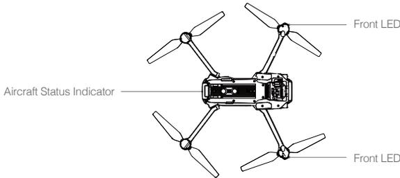
The Front LEDs show the orientation of the aircraft. The Front LEDs glow solid red when the aircraft is turned on to indicate the front (or nose) of the aircraft (the Front LED can be turned off in the DJI GO app). The Aircraft Status Indicator communicates the system status of the flight controller. Refer to the table below for more information about the Aircraft Status Indicator.
