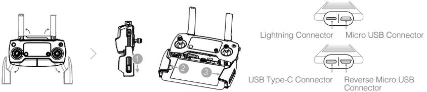
Refer to the figure below for how to replace the RC cable.
