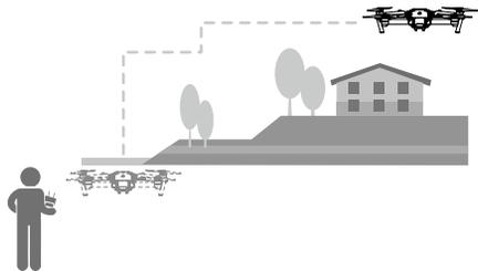
Note that the aircraft will also automatically adjust its speed when it senses there is obstacle at the front of the aircraft or it is flying too close to the ground. However, the user should not rely on this feature to navigate the aircraft between the obstacles. Meanwhile the FailSafe procedure will override the TapFly operation, given that if the GPS signal is weak; the aircraft will exit the autonomous flight from TapFly and fly back to the Home Point automatically.
