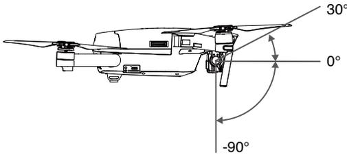
Use the gimbal dial on the remote controller to control camera tilt, or go to Camera View in the DJI GO app, tap and hold on the screen until a blue circle appears, then drag the circle to control the camera's tilt.
