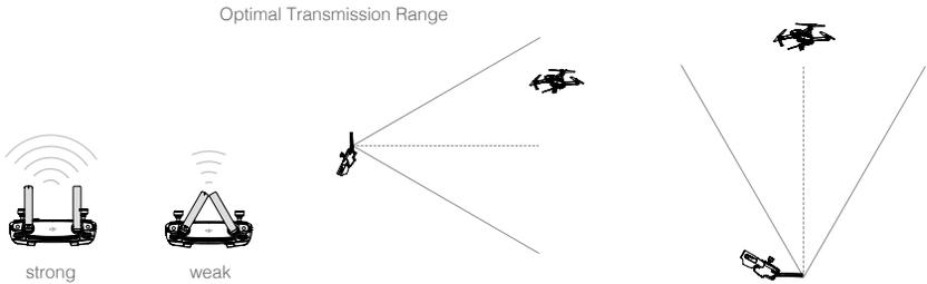
Ensure that the aircraft is flying within the optimal transmission zone. To achieve the best transmission performance, maintain the appropriate relationship between the operator and the aircraft.
