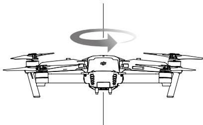
3. Hold the aircraft vertically, with nose pointing downward, and rotate it 360 degrees around the center axis. Recalibrate the compass if the Aircraft Status Indicator glows solid red.
