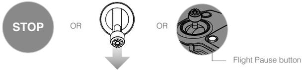
Aircraft will stop and hover after exit from TapFly. You may either tap a new target direction to proceed to the next flight or bring back the aircraft to the Home Point manually.
