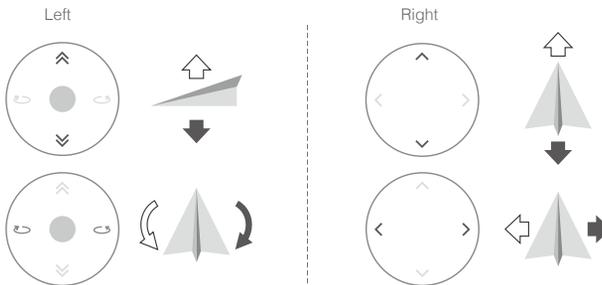
Move the aircraft upwards, downwards or rotate to the left or right by press on the controlling area on the left plane.
