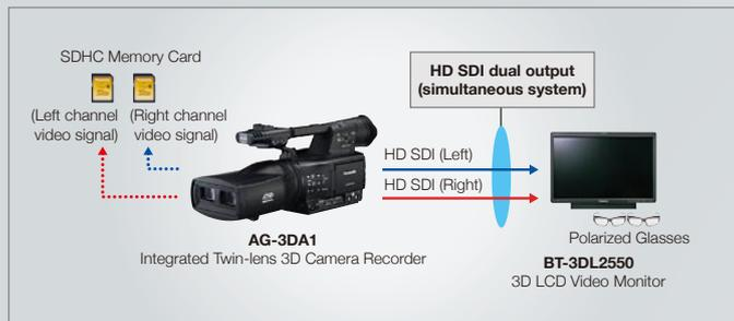
Connecting the BT-3DL2550 3D LCD Video Monitor via HD SDI Dual-Link lets you view the stereo image so that you may adjust the 3D image to create the effect you want by varying the focus and convergence point.
