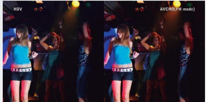
**Sample comparison:** When a flash causes large contrast differences and reduces correlation of consecutive image, HDV shows considerable block noise, while AVCHD in the PH mode minimize break-up.
