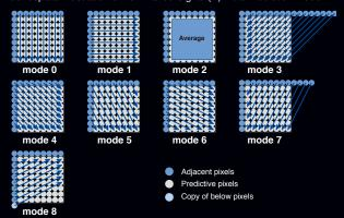
This process generates predictive images based on adjacent blocks of 8  $\times$  8 pixels. Selecting the most suitable predictive mode from among nine luminance signal modes (see illustration) and four color signal modes, it generates accurate predictive images.
