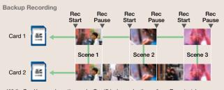
While Card1 record continuously, Card2 independently perform Rec start / Rec pause at Rec trigger.
